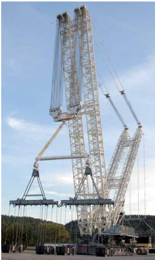
▶▶ The two hook blocks used on the Terex Twin allow the crane builder to use components from the single boom CC8800-1
