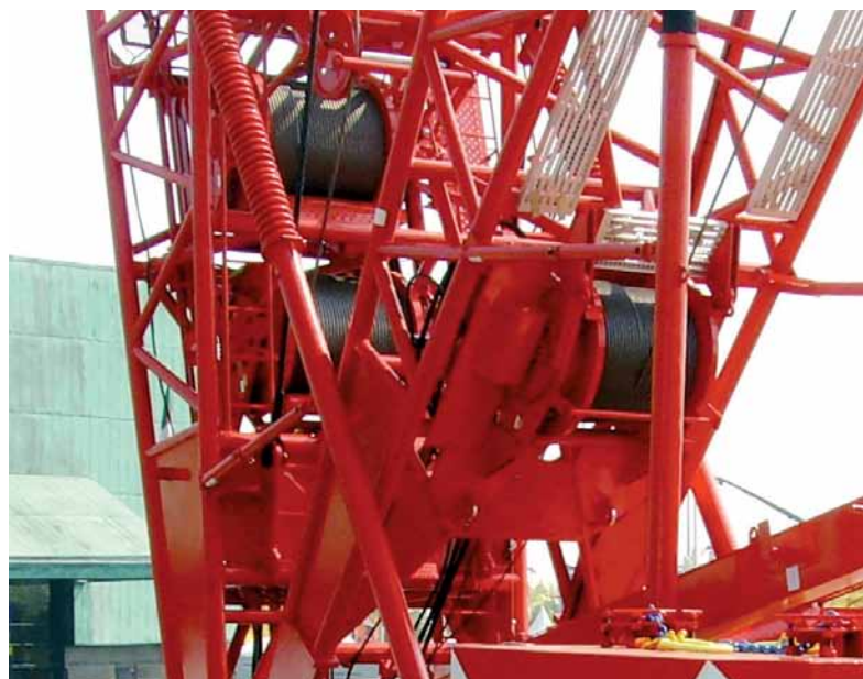
On Kobelco's new SL4500, the rope drum is built into the lower boom section
