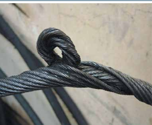
Picture 3: Core or strand protrusion Contact between rope and crane construction points
