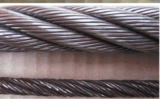
Certex argues that external appearance is not a good indicator of the internal wires. Despite the clean appearance of the outside strands (bottom picture, top), wire breaks were found in the extracted core (bottom picture, bottom) and in the insides of the external strands (top picture)
